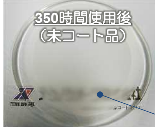
Quartz glass window after 350 hours of use
