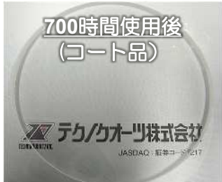
Yttria coated window after 700 hours of use
